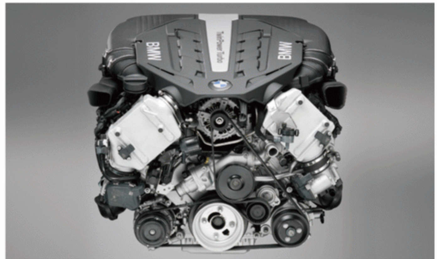
Otto Cycle sample. BMW brand twin power turbo V8 gasoline engine
