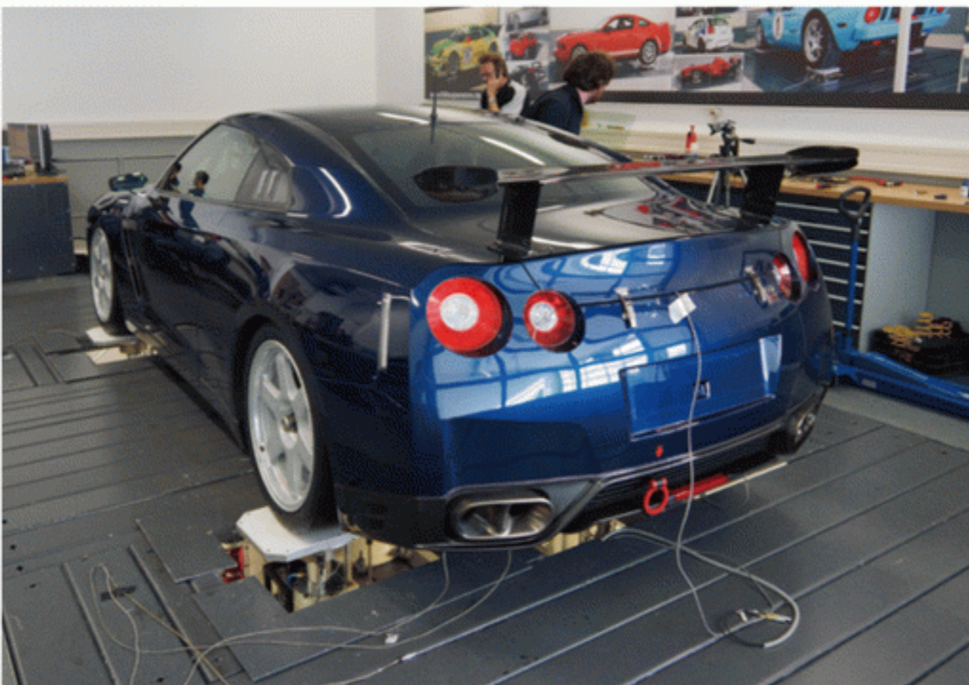
Diagram 1-8-3 Performing the suspension evaluation of the GT-R that participated at the Nürburgring. Testing of the suspension at a variety of vibration frequencies, and analyzing the frequency response
