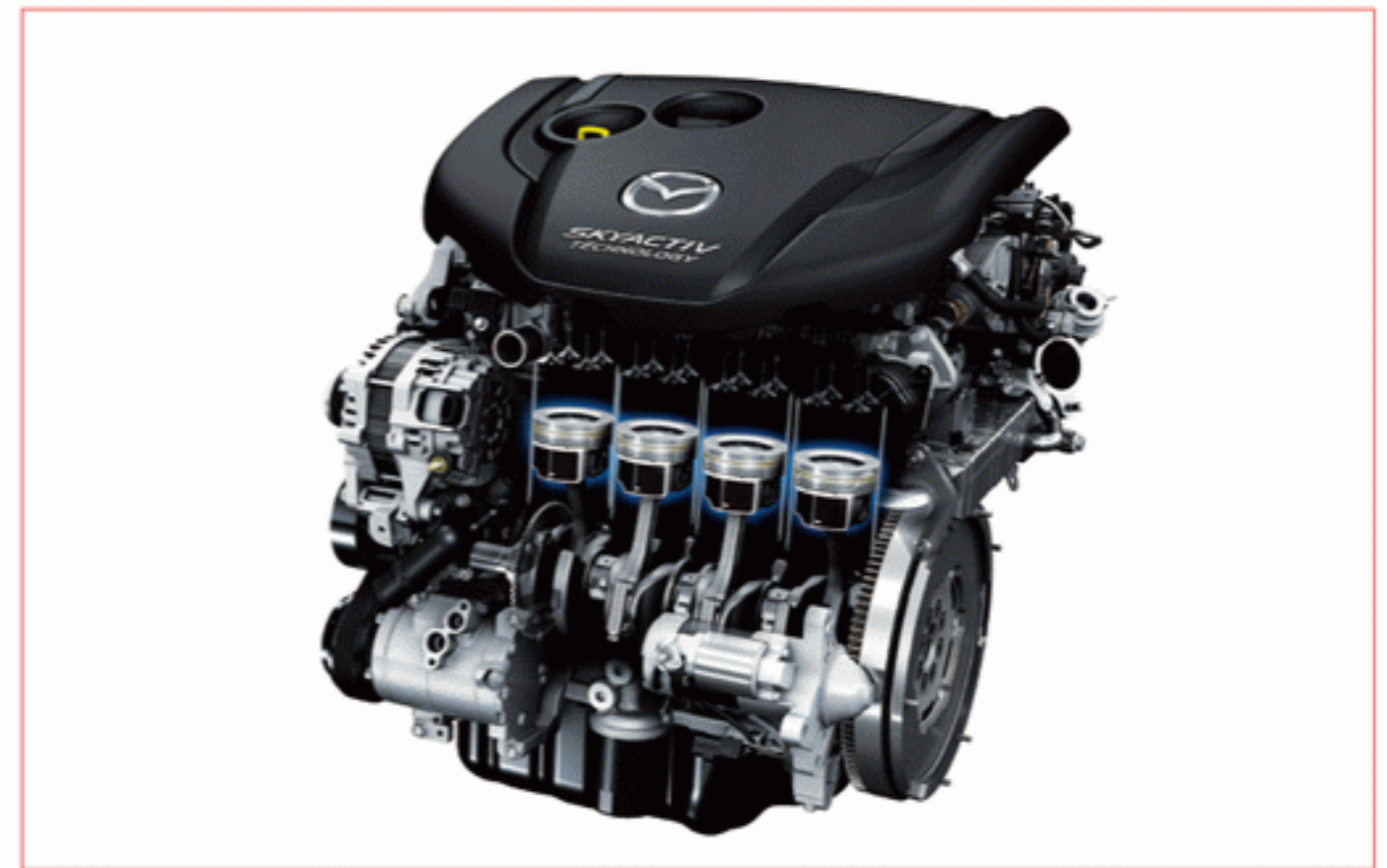
Diesel Cycle sample. Mazda brand 2.2 liter Diesel engine
